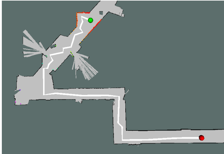
Figure 3: Example path planned by the RRT algorithm in Stata basement, with a padding size of 0.25 meters. The green and red markers represent the start and goal respectively, while the white line represents the planned path.
